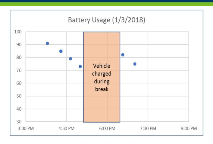
Jan. 3<sup>rd</sup>, 2018 Battery Charge Readings Start Temp.: 3° F; (-13° F windchill); Wind: WNW 11 mph
