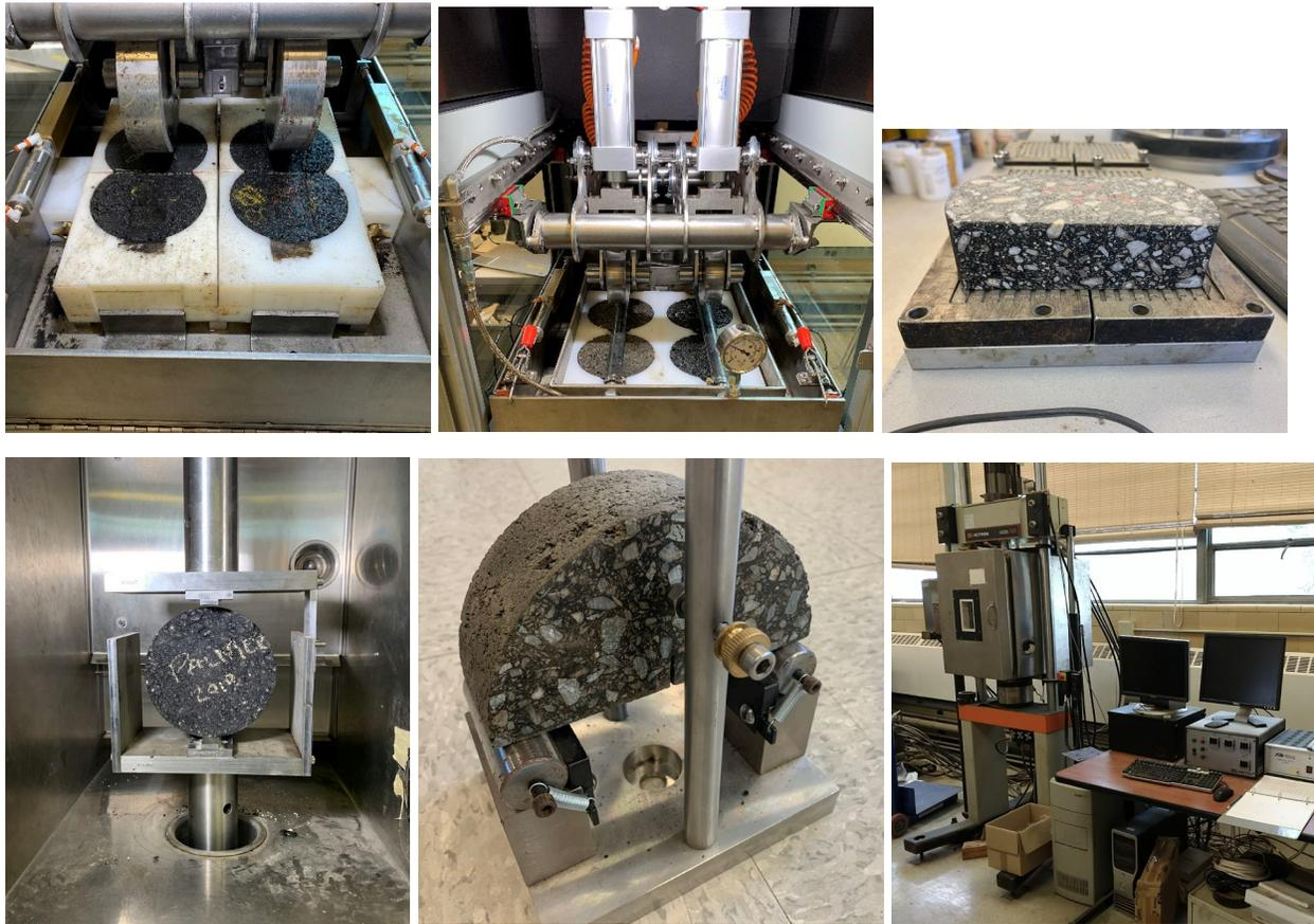
**Figure 4-2 Mixture Performance Testing conducted at the CAP Lab in preparation for Balanced Mix Design Implementation. Clock-wise from the top-left corner: Hamburg Wheel Tracker (AASHTO T324), Asphalt Pavement Analyzer (AASHTO T340), Texas Overlay Test, 100 Kn Instron 1331 Load Frame with FastTrack 8800 Data Acquisition System, SCB-FIT Test (AASHTO TP-124), IDEAL CT Cracking Test (ASTM D8225)**
