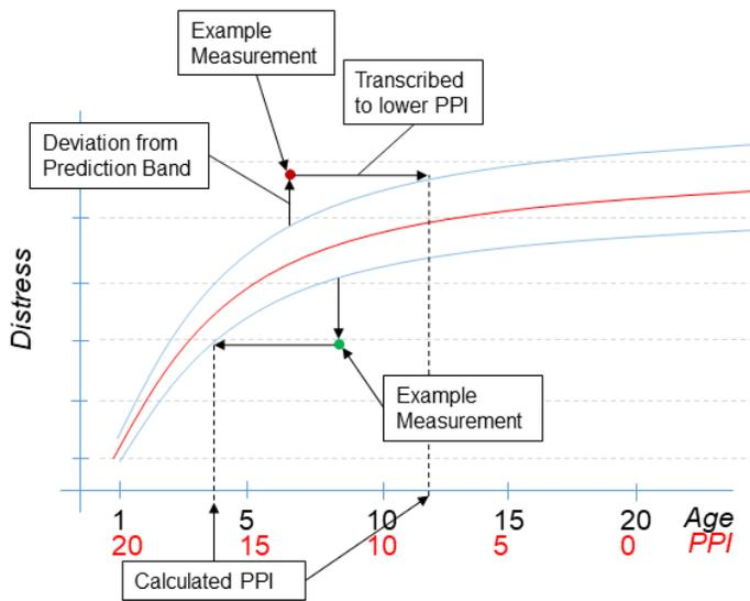
**Figure 2-10 Concept Level Graphic for PSPI Model Determination**
