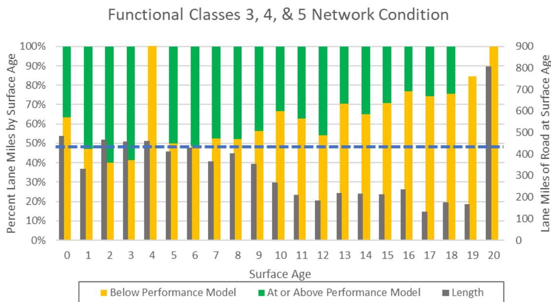
**Figure 2-13 PSPI Ranking at or above projected condition level vs. age for Functional Classes 3, 4, and 5**
