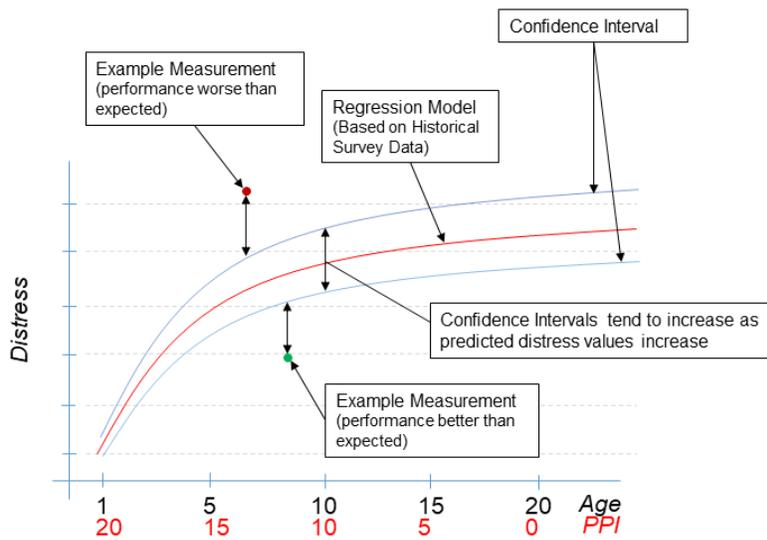
**Figure 2-9 Concept-Level Graphic for PSPI Model Prediction**
