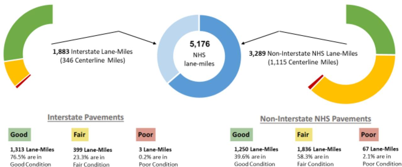
**Figure 2-15 Connecticut NHS Pavement Inventory and Conditions as Required for FHWA Reporting (Based on 2020 HPMS pavement condition data submitted to FHWA June 14, 2021 )**
