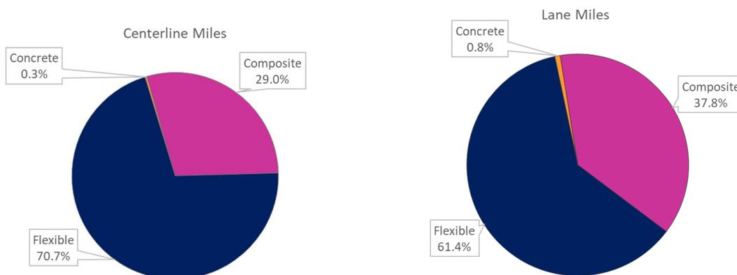
**Figure 2-3 Distribution of CTDOT Pavement Network Surface Type by Centerline and Lane-Miles**
