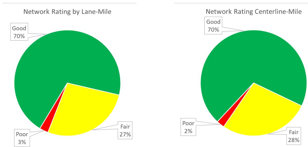
**Figure 2-6 Conditions of CTDOT-Maintained Roadways (2020) Using the PCI, by Lane Mile and Centerline Miles (Excludes Town Roads + Overlapping Routes)**
