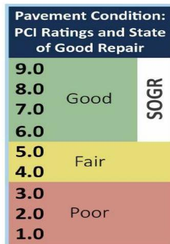
**Figure 2-4 PCI Ratings used to define SOGR and Pavement Condition**
