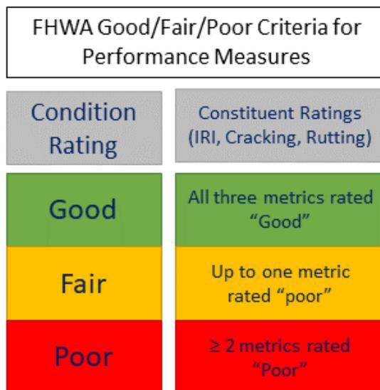
**Figure 2-14 FHWA Performance Measure Criteria for Good/Fair/Poor Ratings**
