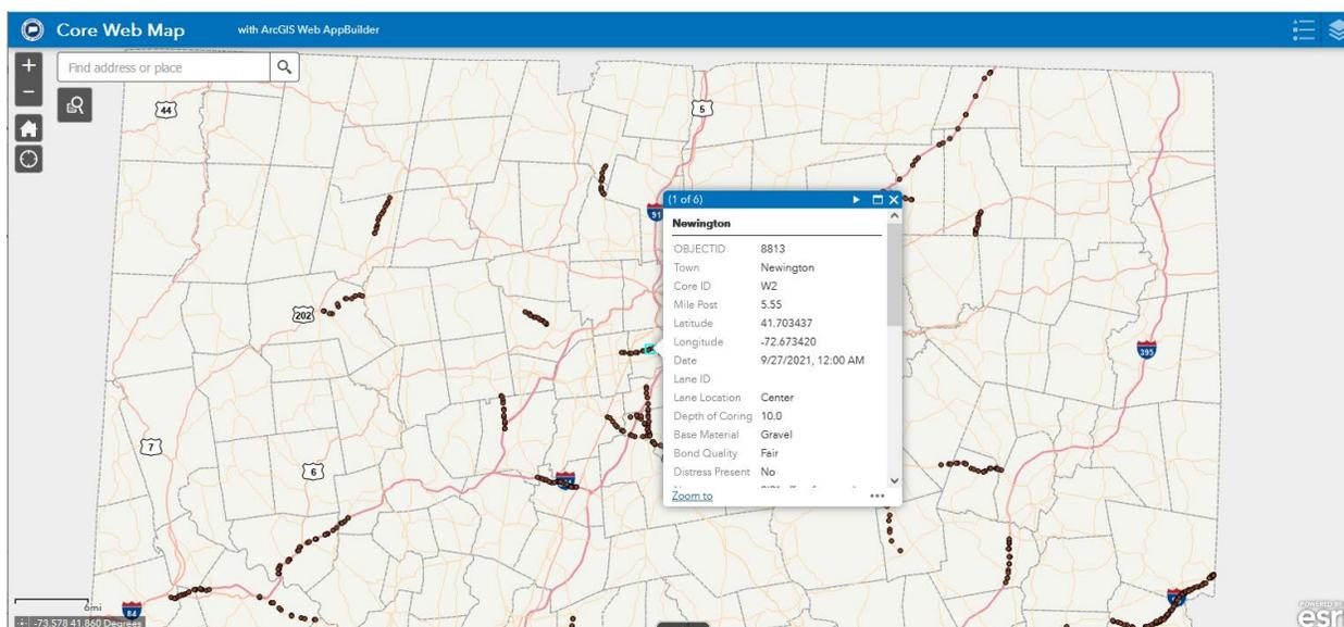
**Figure 4-3 Core Database for State-wide Forensic Pavement Coring in the TED/GIS Interface**
