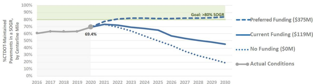
**Figure 3-3 Connecticut Pavement Performance Projections for the CTDOT Maintained Network (from May, 2020 CTDOT Asset Fact Sheet)**
