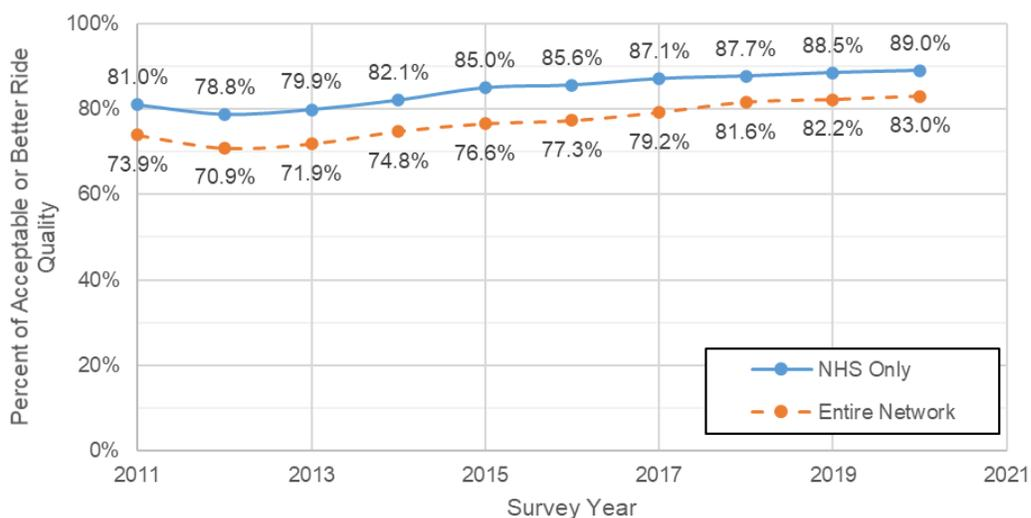
**Figure 2-16 Ride Quality (IRI) Using 3-year Moving Average for the NHS Systems, and the Entire CTDOT-maintained Network, for Calendar Years 2011 through 2020.**
