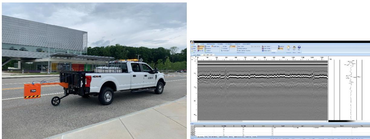
**Figure 4-1 CAP Lab vehicle with the 2.0 GHz Air-Launched RADAR (left), Software output showing radio signal of GPR data (right)**
