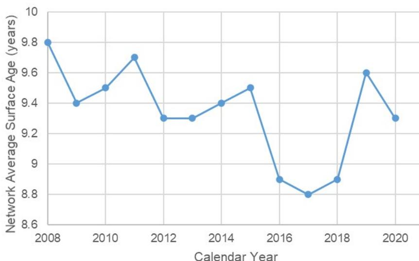
**Figure 2-2 CTDOT-Maintained Network Average Surface Age Over Time (2008-2020)**
