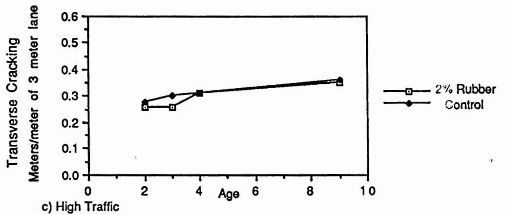
Figure 22. Transverse Cracking versus Age, 2% Rubber, Medium Distress
