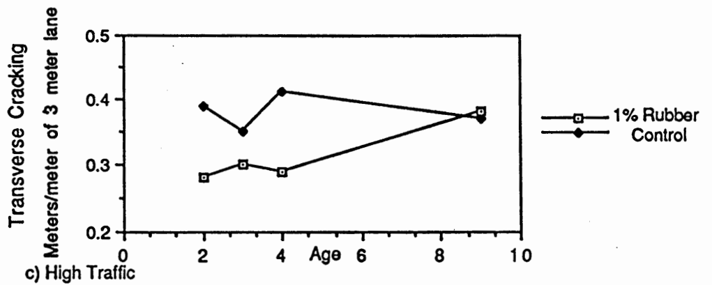
Figure 9. Transverse Cracking versus Age, 1% Rubber, Medium Distress
