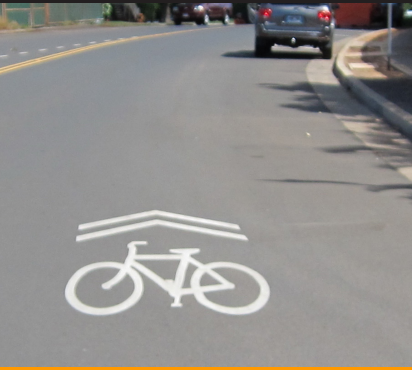
SHARED LANE MARKING
