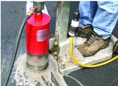
In cooperation with ConnDOT and FHWA, the CAP Lab conducted a two-year study using a nuclear density gauge to compare the in-place density of asphalt pavements with the density of cores cut from the pavement. The research has generated a procedure for establishing a correction factor used to adjust the nuclear density gauge readings of in-place asphalt to more closely approximate the densities found in cut cores.
