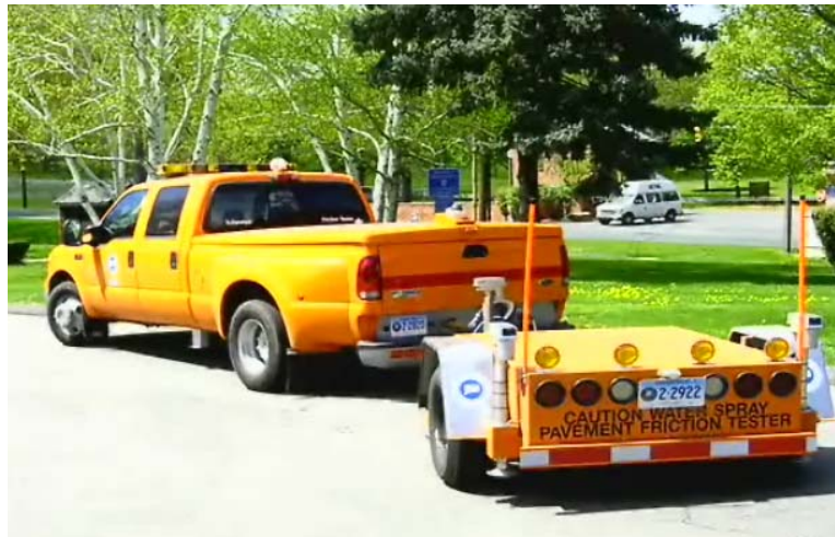
Figure 2-2. ConnDOT Friction Tester.
