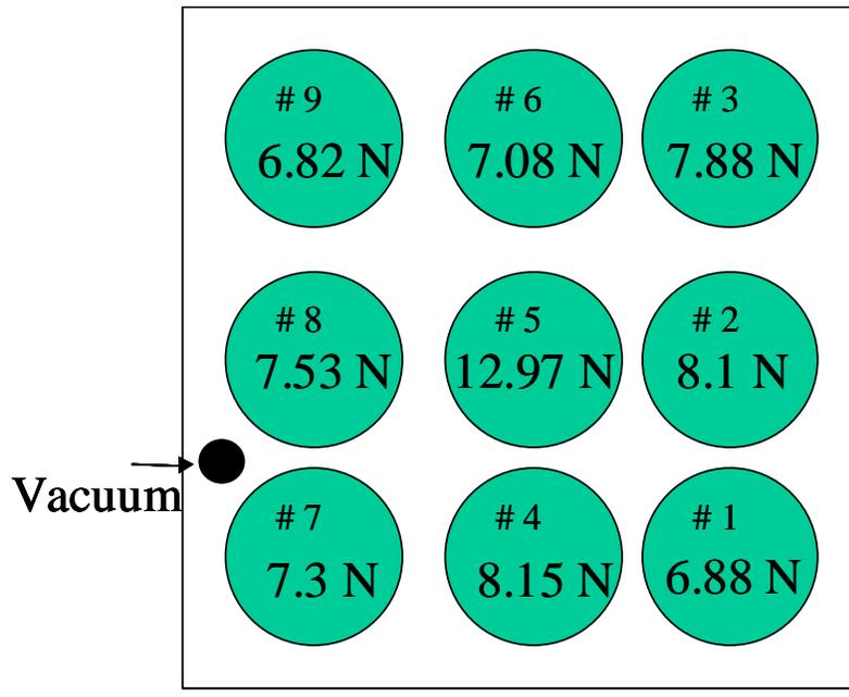
**Figure 4.** Force calibration. (A) Photo of silicone samples in the center of wavy washers being squeezed in the combinatorial rheometer for force calibration; and (B) resulting forces with a pressure difference of 90 kPa across the membrane.
